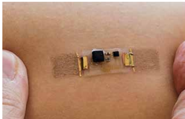
Epidermal bærbar sensor. University of Illinois, USA
